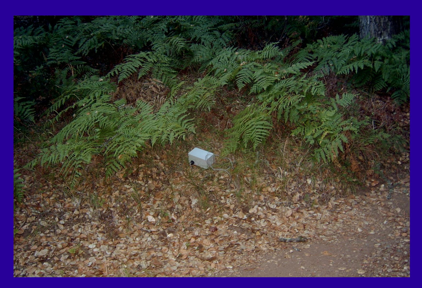
The US Geological Survey (USGS) currently monitors the temperature of various parts of Yellowstone National Park. At their request, we are designing a wireless sensor network which will automatically record and upload temperature readings to a server. This sensor network must be low power, failure tolerant, long-range and survive under adverse environmental conditions.
